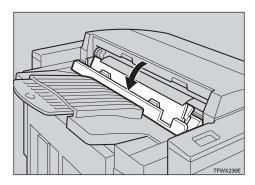
Push the front cover release button and open the front cover.
